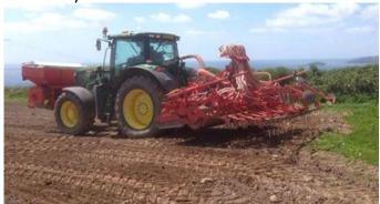
Planted with a power harrow drill combination mounted on tractor that steers itself using GPS. Using modern technology for the benefit of the environment.
